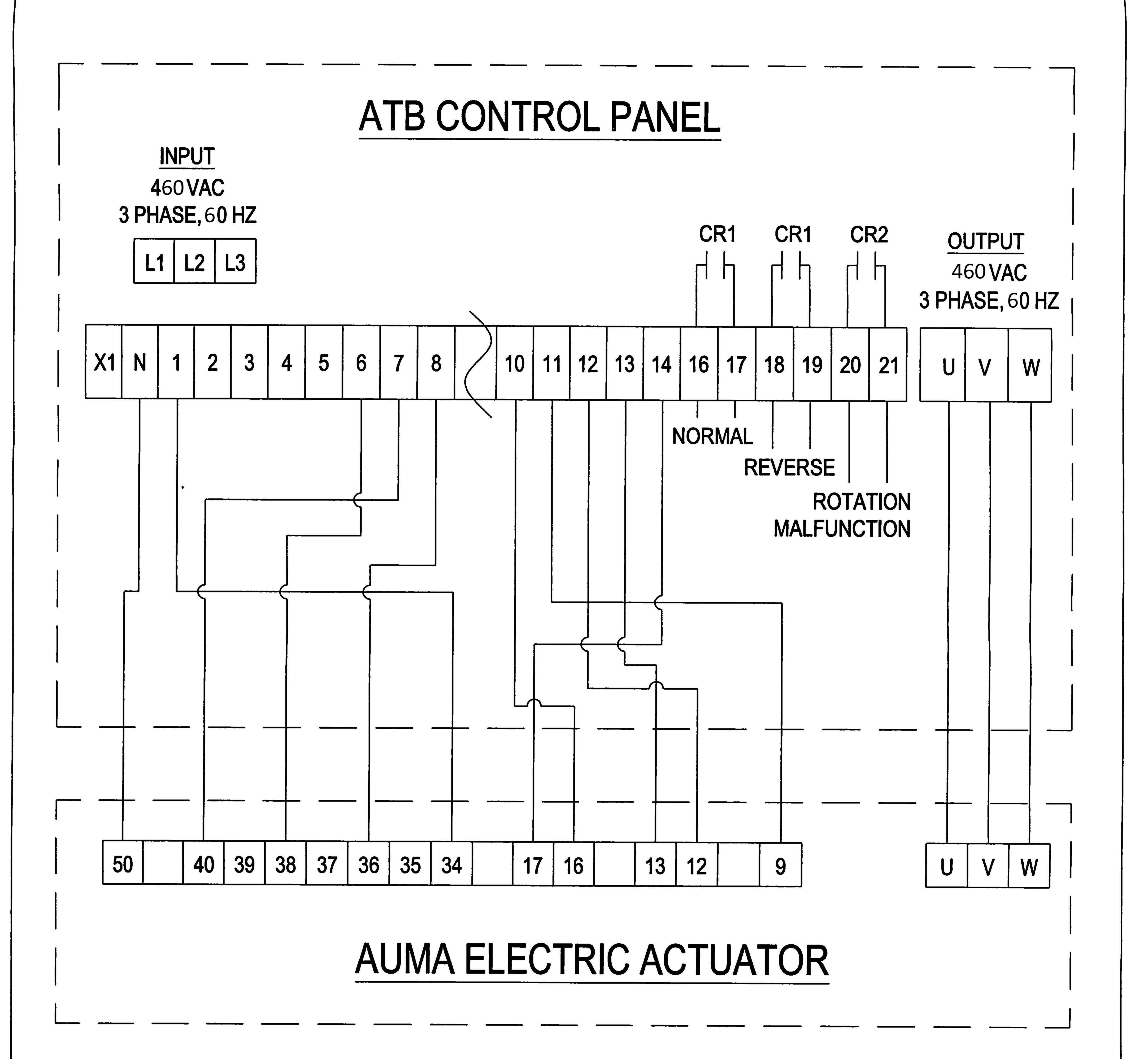
NOTE: AUMA factory wiring in AUMA cap sometimes comes from AUMA with a Jumper installed between terminals 17 and 49, but it should be installed between terminals 18 and 50 (with another Jumper installed between 34 and 49).
