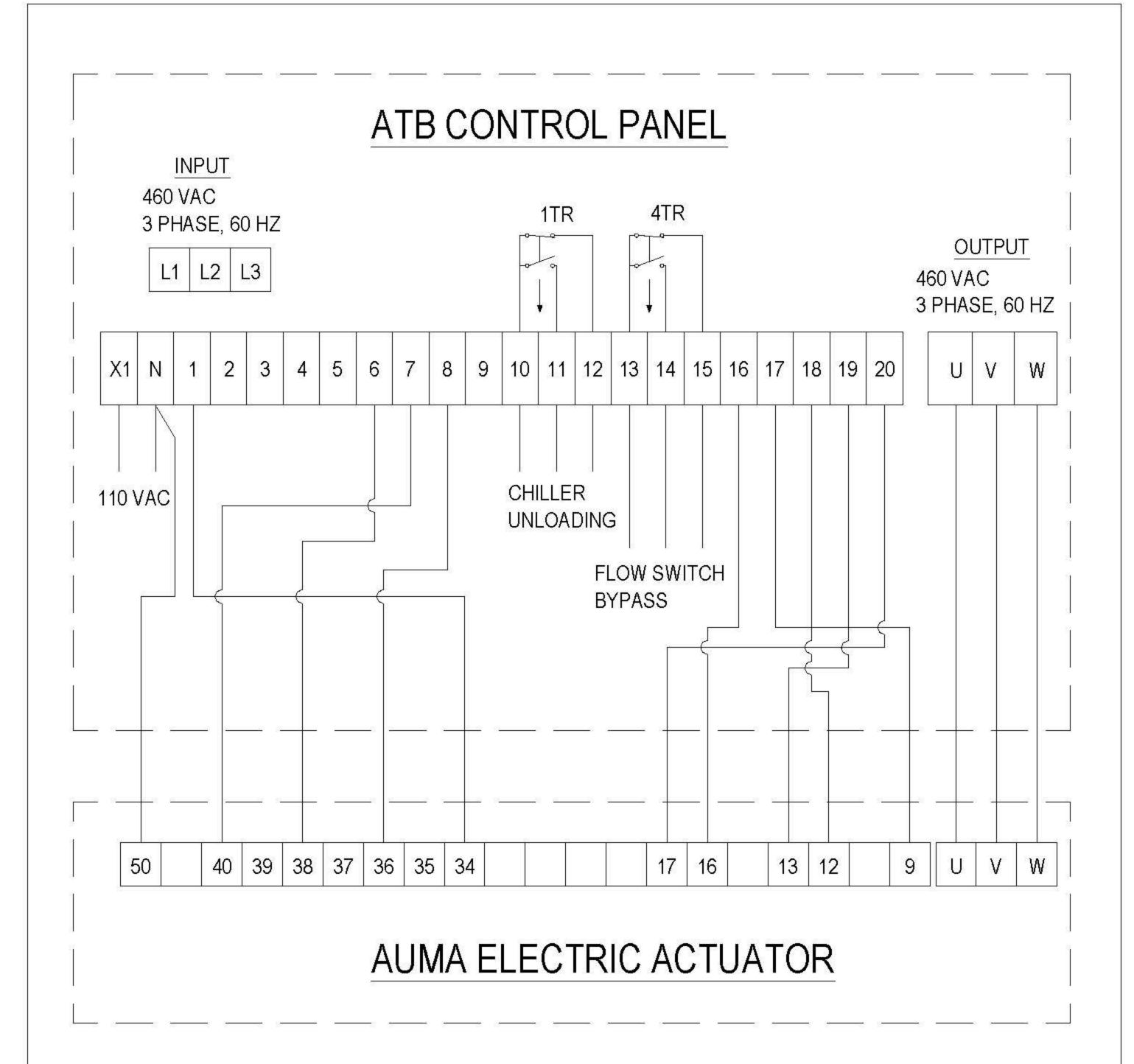
NOTE: AUMA factory wiring in AUMA cap sometimes comes from AUMA with a Jumper installed between terminals 17 and 49, but it should be installed between terminals 18 and 50 (with another Jumper installed between 34 and 49).
